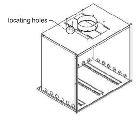
Refer to the diagram and table below to determine which hole to use for your heater.
