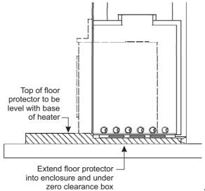
The heater may be <u>elevated</u> and installed so that the <u>base</u> <u>of the heater is above the floor</u>. The height at which the heater is installed will determine:
