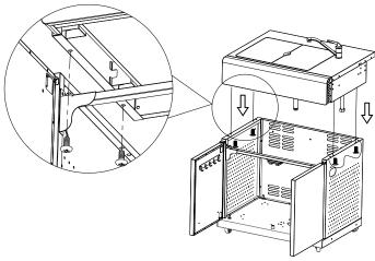
Fit the cover plate to the base shelf of the cart to cover the cylinder hole.
