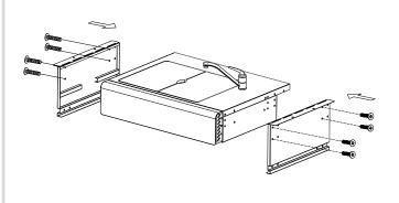
Use help to carefully fit the sink unit into your build-in construction.
