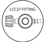
GAS HOSE Regulator connection (to ULPG cylinder)
