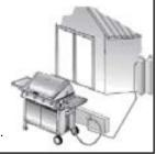
If using a flexible hose connection, attach the safety chain (Item# 29) shown on part diagram (page 10) to a strong point at the bayonet connection point and to the right-hand side of the bottom shelf of the barbeque. This is to prevent the flexible hose from being stretched and becoming damaged.
