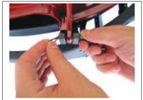
Lock the hood into place by fitting a hinge pin through the firebox flanges and the hood hinge arms on each side. Fix the hinge pin by inserting "R" clip through the end of each pin.
