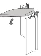
Loosen the bolts on the remaining brackets; you do not need to remove these brackets. Lift the bracket up and rotate sideways and remove the firebrick.
