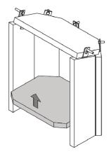
Lift the top firebrick slightly to get access to the bracket and bolt for the side brick, as shown. Remove the bracket a n d the side firebrick.
