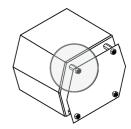
Fit the base and mounting post assembly to the base of the firebox with four small silver bolts and nuts supplied, with the nuts being on the underside.
