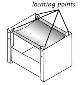
Locate the column onto the four locating points on the base of the heater. For the Forester and the Legend, the side of the column with a 45 mm gap on the bottom edge goes at the rear of the heater. For the Nevada, the side of the column with the 10 mm gap goes at the rear of the heater.
