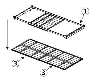
STEP 2: ATTACH PART ③ TO PART ① USING BOLTS AS SHOWN BELOW.
