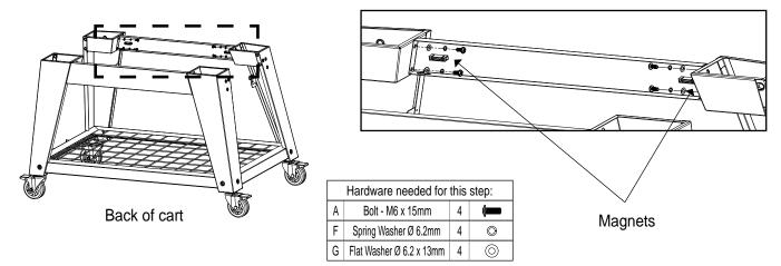
Ensure rail is attached with 4 bolts, spring washers and flat washers. Don't fully tighten yet.
