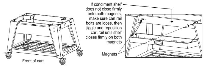
c) Once the shelf is closing firmly on both magnets, KEEP THE SHELF CLOSED and firmly tighten the cart rail bolts you inserted in Step 6. **Tighten all bolts firmly.**
