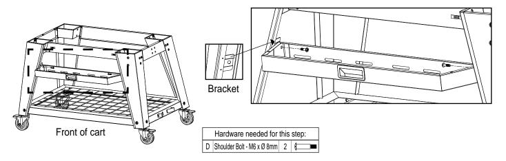
Ensure condiment shelf is attached with a bolt on each side.
