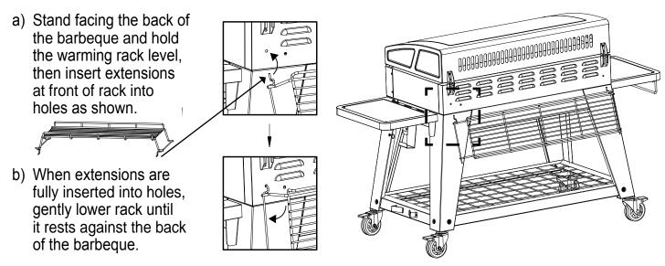
NOTE: When the barbeque is not in use, it is NOT recommended to store the rack on the back of the barbeque unless it is stored in a dry, covered area.
