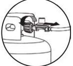
B. To disconnect cylinder, turn end of hose in an anticlockwise direction
