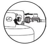
A. To connect cylinder, screw end of hose tightly onto cylinder in a clockwise direction.
