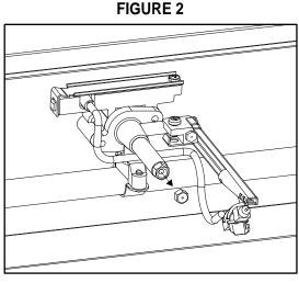
Valve with LPG injector removed (ensure natural gas injectors remain attached and re-tighten if necessary)
