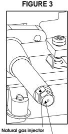
Natural gas injector (behind LPG injector)
