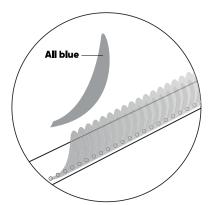
B. Incorrect - all blue flame and noisy operation (e.g. popping) indicates that burners need cleaning or replacing
