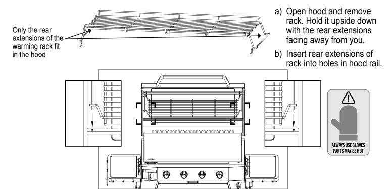
NOTE: To avoid damage to rack or hood, <u>ALWAYS REMOVE</u> rack from hood storage position before lighting barbeque, or when cooking.
