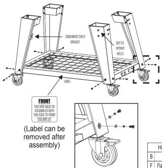
**NOTE:** Legs must be assembled correctly to cart bottom shelf by identifying front of shelf, and front legs.
