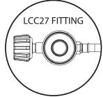
GAS HOSE Regulator connection (to ULPG cylinder)
