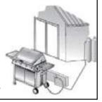
If using a flexible hose connection, attach the safety chain (Item# 27) shown on part diagram (page 10) to a strong point at the bayonet connection point and to the right-hand side of the bottom shelf of the barbeque. This is to prevent the flexible hose from being stretched and becoming damaged.
