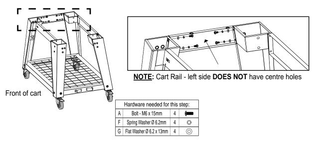
Ensure rail is attached with 4 bolts, spring washers and flat washers, and tighten all bolts firmly.
