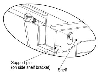
d) Select right side shelf and rest it on the shelf shelf brackets attached to the right side of the cart assembly. Repeat steps b) and c) to fasten right side shelf to the cart assembly.
