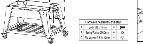
Ensure gas cylinder hook is attached with 4 bolts, spring washers and flat washers, and tighten all bolts firmly.
