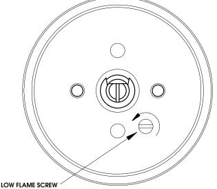
Turn 3.5 turns (1,260° to fully open valve for natural gas use)
