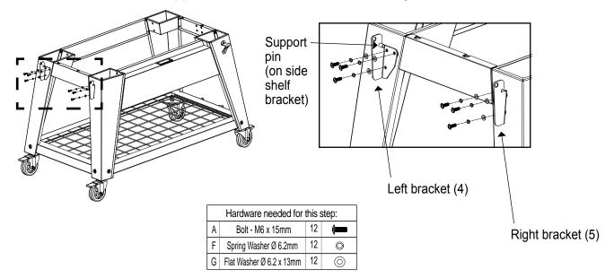
Ensure each support is attached with 3 bolts, spring washers and flat washers, and **tighten all bolts firmly.**
